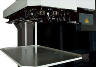
Change up to 20/40 electrodes Supports continuous machining using many electrodes
