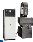
DM250+DE30T Transistor pulse power supply Began shipment in Feb. 1967
