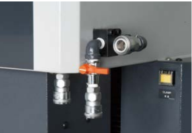
Sprays dielectric fluid between the workpiece and electrode during pitch machining
