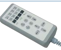
LCD display improves workability Workpiece coordinates can be set from the manual operation box The jog feed rate can be changed between 50 and 150% using the override function
