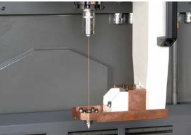
Supports fine-hole machining, and fine-hole jig is removable
