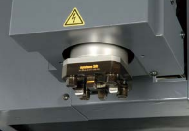
Supports parallel electrode setup and index machining Supports fluid emission from spindle center (photo shows 3R-MACRO chuck specifications)
