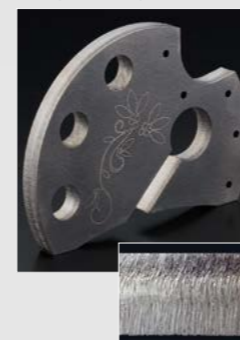
Mild steel (SS400) t9mm Nitrogen cutting
