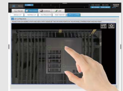
By superimposing the program shape on the converted image, positioning and workpiece placement for off-cut materials can be intuitively performed.
