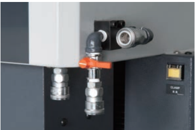
Sprays dielectric fluid between workpiece and electrode during pitch machining.
