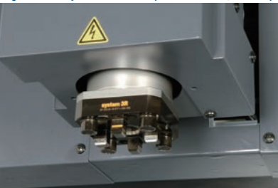
Highly accurate helical machining and index machining are possible Compatible with fluid emission from spindle center (photo shows 3R MACRO chuck specifications)
