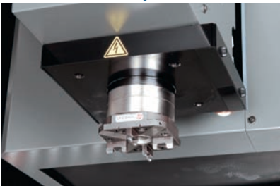
Clamp spindle side holder with air chuck (photo shows EROWA ITS50 chuck specifications)
