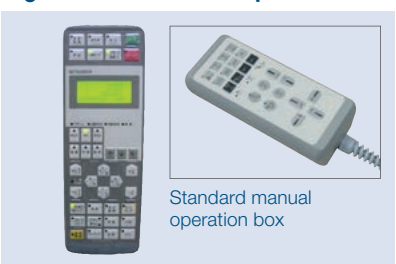
LCD display improves workability. Workpiece coordinates can be set from manual operation box. Jog feedrate can be changed between 50 and 150% with override function.
