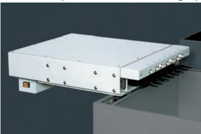
Change up to seven electrodes (only Combi specifications) Compatible with continuous machining using multiple electrodes
