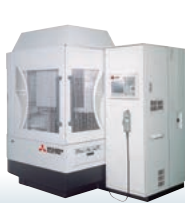
2001 MA2000 Began shipment in May 2001 Equipped with thermal displacement compensation
