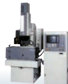
1986 M25KC4 Began shipment May 1986 Equipped with ultralow-wear power supply (slope control system)
