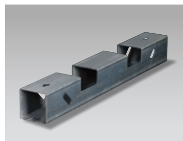
t1.6mm mild steel (assist gas: oxygen)
