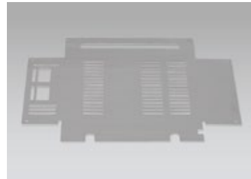
t1.0mm steel (assist gas: oxygen)
