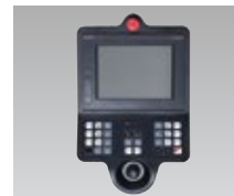
✓ Teaching Panel with Joystick The joystick allows for intuitive axial movement.
