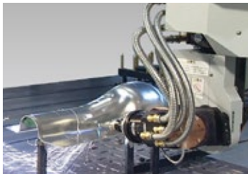
t3.0mm aluminum alloy (assist gas: air)
