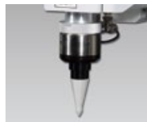
✓ Teaching Sensor Used to teach points automatically by pressing the tip pin against the work piece.
