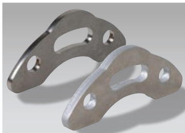
Left: t6mm stainless (assist gas: nitrogen) Right: t8mm aluminum (assist gas: air)
