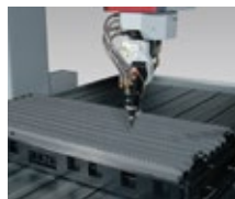
✓ 2D sheet processing pallet Equipped with manual clamps and scrap drawer.
