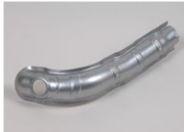
t0.5mm plated steel (assist gas: air)
