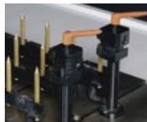
✓ Work Support Pins and Clamps Supports 2D work pieces.
