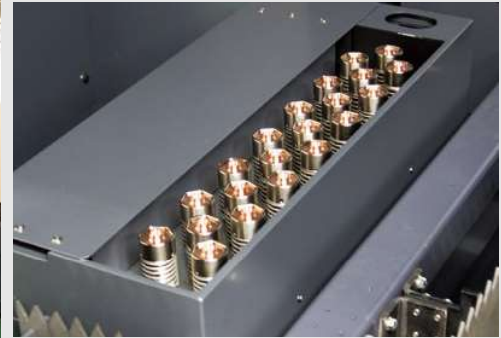
Automatic replacement of a defective nozzle. Accommodating up to 21 nozzles, this technology supports prolonged continuous processing.
