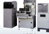
1979 DWC90-CNC1 Max. machining speed 60mm 2 /min
